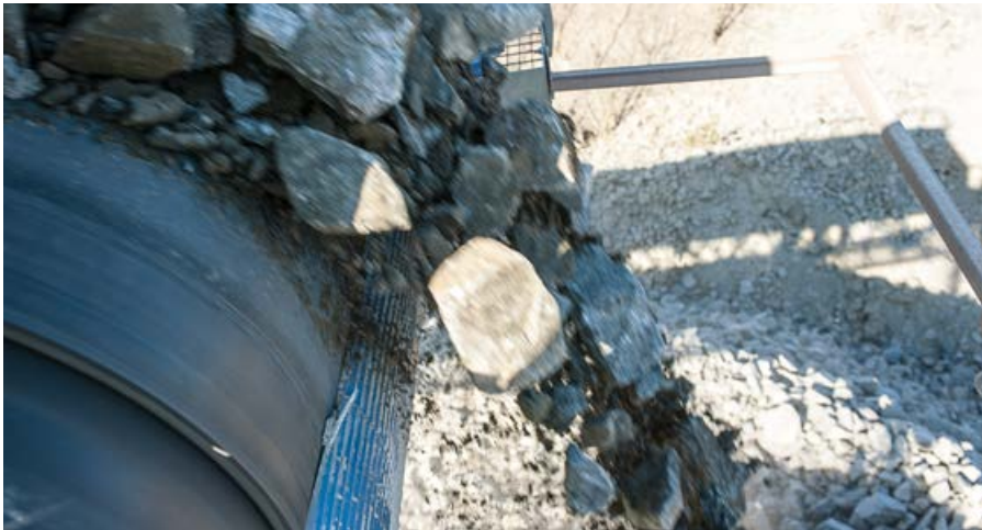
In the majority of cases, the primary belt cleaner is positioned on the head pulley, which is where the material leaves the belt.
